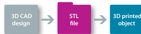
Figure 4: An STL file serves as the bridge between 3D CAD designs and 3D printer hardware
